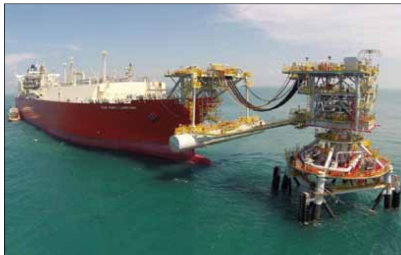
▲ PGN FSRU Lampung was Indonesia's second floating regas terminal and the first to use a tower yoke mooring system.
